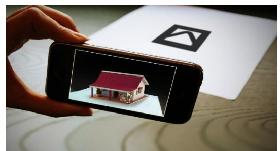
Fig. 2. Marker-based Augmented Reality
